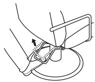
With the seat in the desired orientation, hold the chair top and raise up the foot pedal to lock the seat so that the chair top will not turn.
