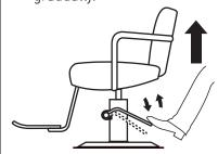
Note: Be careful not to press down the foot pedal too deeply. The seat will go up but also down, resulting in only a slight rise. (2) Lowering the seat
