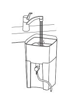
(2) Water receptacle must be placed lower than TJ-6. Open the valve, and purified water comes through plastic tube into the receptacle. Keep the water tank covered except when pouring tapped water into the tank.
