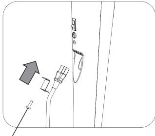
1 pan head screw, M3 x 15 (with a flat washer and a spring washer)
