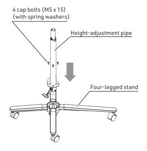
Insert the height-adjustment pipe into the four-legged stand. Loosely attach them together with the four screws provided.
