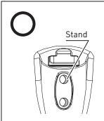
When you slide the upper main unit, the screw holes become open or closed. (The screw holes are open when those in the main unit align with those in the stand.)
