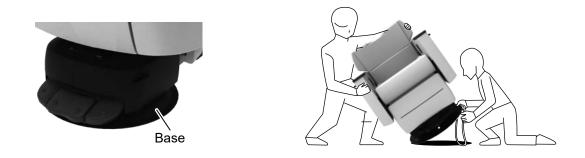
During installation, ensure that the power cord outlet of the chair base is aligned with the chair front. Failure to follow this instruction may cause damage to the power cord.
