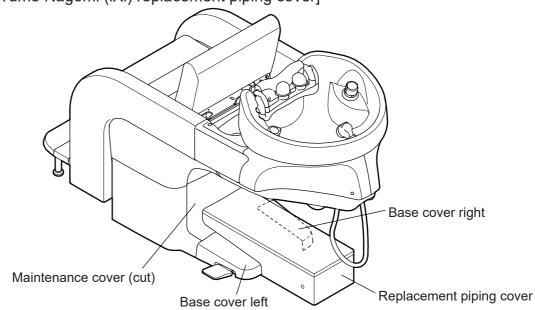
Note: This instruction Instruction is a supplementary instruction that is used only when replacing Rear Shampoo or NRS wash unit with Yume Nagomi (iXi) wash unit. Follow the "Yume Nagomi (iXi) Installation Instruction" for installation of the wash unit.
