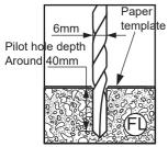
(1) Drill a pilot hole to the specified diameter and depth.
