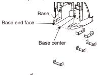
\*When the above floor plumbing cover C is cut and then used, the number of floor-anchor fittings to be used varies.
