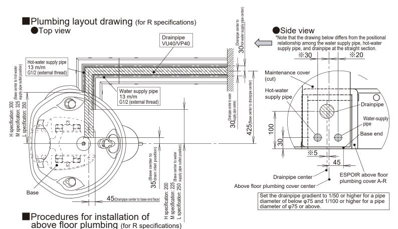
(1) Temporarily place the floor-anchor fittings on the floor by referring to "Floor-anchor fitting installation positions." At this point, determine the floor-anchor fitting positions with reference to the base center and base end face.
