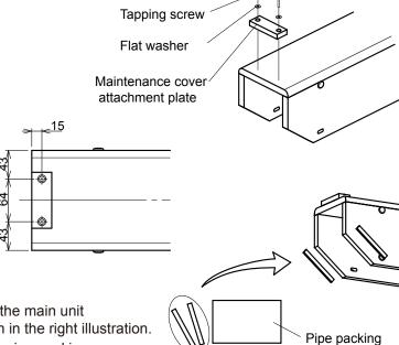
\* Double-sided tape is originally applied to the pipe packing.
