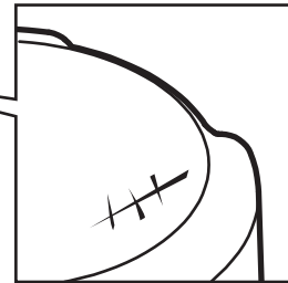
Example of scratches on the plated surface
