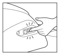
■ The power switch is located at the left side of the base. The power turns ON if the right side (I mark) is pushed, and turns OFF if the left side (○ mark) is pushed.
