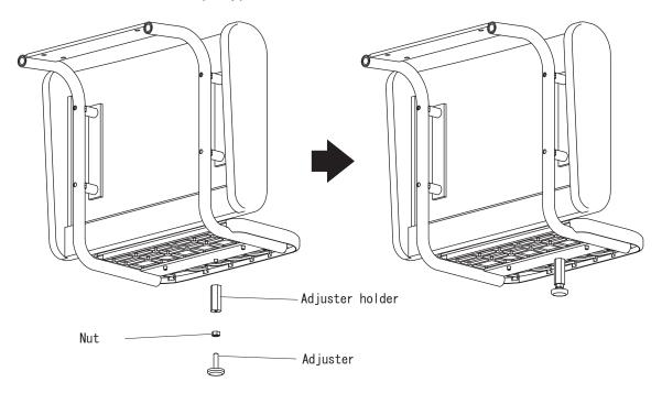
Attach the step adjuster as per the above illustration. The parts to use and the attachment distance should be referred to the below.
