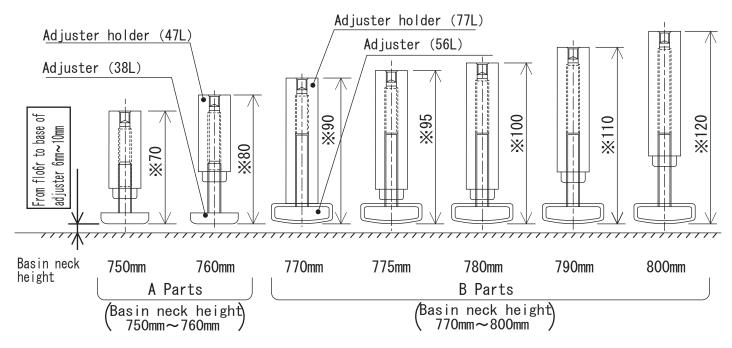
(Note) In the case of 770mm neck height, remove the nut and tighten the adjuster to use.
