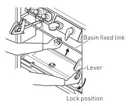
7 Insert the basin straight into the basin body parallel, with keeping the clearance between the basin and the operation panel.
