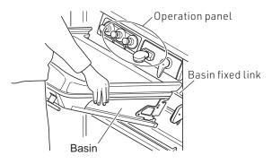
\* When the lever is set in the free position, lift the basin fixed link and turn the lever to the lock position.
