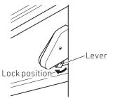
4 Hold both ends of the basin. Lift the front side of the basin slightly and pull it out.
