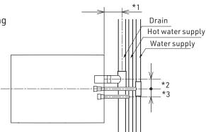
Make sure that the drainpipe does not have double trapping. CAUTION Drain failure or abnormal noises may occur.
