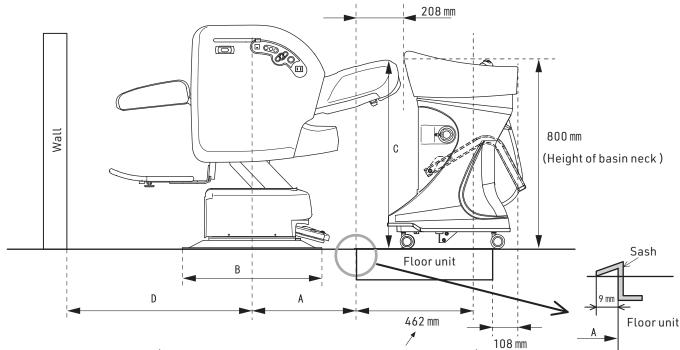
(Distance from center of drain port to front end of floor unit)
