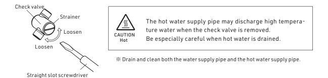
5 Drain and clean both the water supply pipe and the hot water supply pipe.
