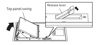
4. Remove the maintenance lid and insert it into the gap of the opened top panel swing .
