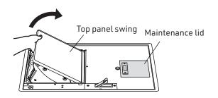
5. Hold the opening generated by removing the maintenance lid and lift the top panel upward.
