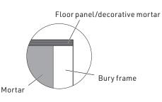
When wood flooring or tiles are used around the openings, select a material equal to or thinner than 12 mm. Otherwise, the floor unit cannot be secured.
