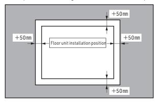
%Cut the panel + 50 mm larger around the attachment position.
