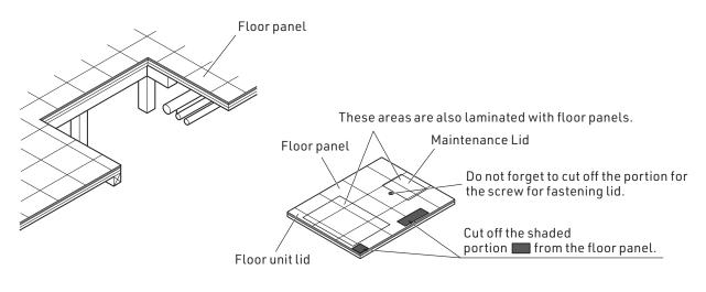
%Be sure to cut off in an exactly same shape as the cut window.
