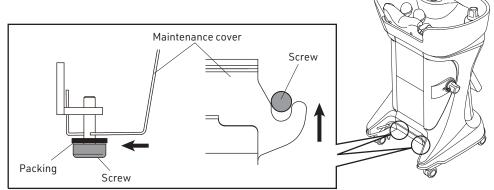
1. Loosen the screws (two positions: left and right)
