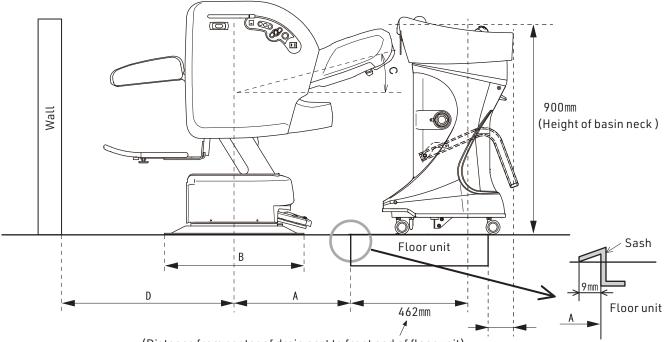
(Distance from center of drain port to front end of floor unit) 108mm
