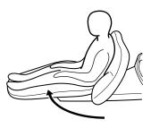
4 Press the P1 switch (or manual mode control) to bring the chair to its approximate position.
