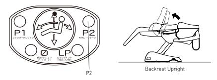
2 Press the lock position switch to unlock the chair rotation.
