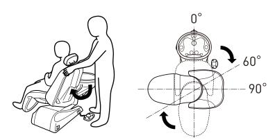
4 Press the lock position switch to lock the chair rotation.
