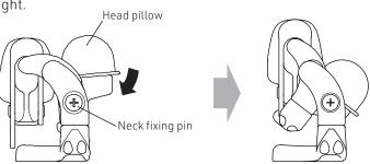
② Push out the neck fixing pin, and turn it clockwise to lock.
