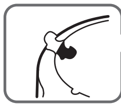
An example of peeling on the plated surface
