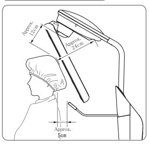
Place the top of the head approximately 12 cm away from the pivot of the ring and approximately 24 cm away from the infrared thermal sensor.
