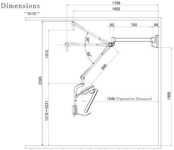
$\ast$  The above shows reference values when the lower end of the wall mount plate is installed at a height of 1900 mm from the floor surface.
