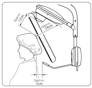
Place the top of the head approximately  $12~\mathrm{cm}$  away from the pivot of the ring and approximately  $24~\mathrm{cm}$  away from the infrared thermal sensor.
