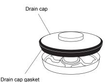
The drain cap is a consumable supply. When water stored in the basin drains faster due to its deterioration etc., replace it (on a chargeable basis).
