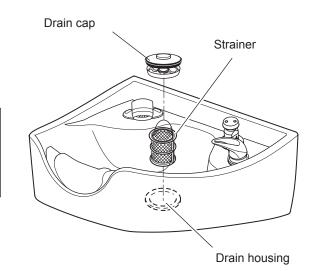
3 Install the strainer in the drain housing.(stPush firmly so as not to float)
