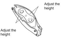
5. Insert and secure the neck fittings to the neck base. Pay attention to the proper direction of neck fittings.The surface of neck cushion with cutaway to be faced to the chair side. 2. Hold the neck cushion, and fit it to the centre of neck fittings.
