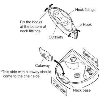
Do not force the neck cushion if it does not fit smoothly. Instead, check the following points. Forcing the neck fittings on may cause damage to the neck base or injury to customers.
