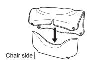
4. While pulling the neck cushion, secure it with the hooks (2 locations). As shown in the below illustration, secure the hooks at the bottom of neck fittings.
