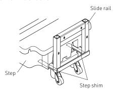
3 Attach the two locations on the top of the step slide rail to the basin unit using truss-head screws. (M6 x 15, 2 screws)
