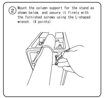
Mount the stand base on the column support as shown below, and secure it firmly with the furnished screws using the L-shaped wrench. (4 points)
