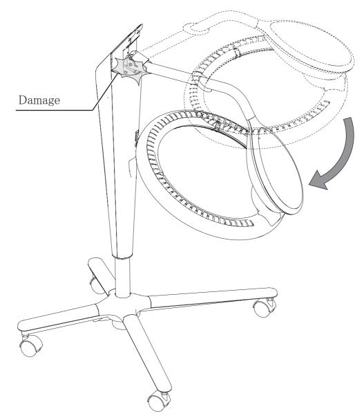
Do not apply pressure onto the shaft. \*Doing so may cause a damage of the product.
