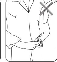
Hold the shaft firmly with your hands throughout the procedure of step. Never release your hands from the shaft until you complete tightening the screws.
