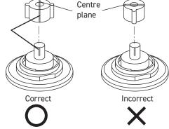
3. Attach the thermostatic control knob to the conversion adaptor, and fix it with the screw.
