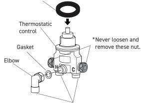
Attach the elbow in the same direction as the flexible pipe connecting port.
