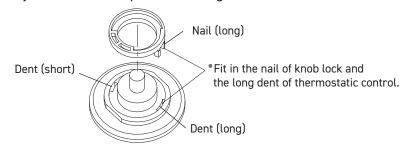
${\bf 2}.$  Attach the conversion adaptor to the thermostatic control.
