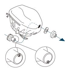
1 Attach the cap joint N to the mist cap (option).
