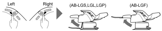
⇒ If any switch except for the legrest heater switch is pressed while the chair rotation lock is released, chair rotation is engaged and then locked.
