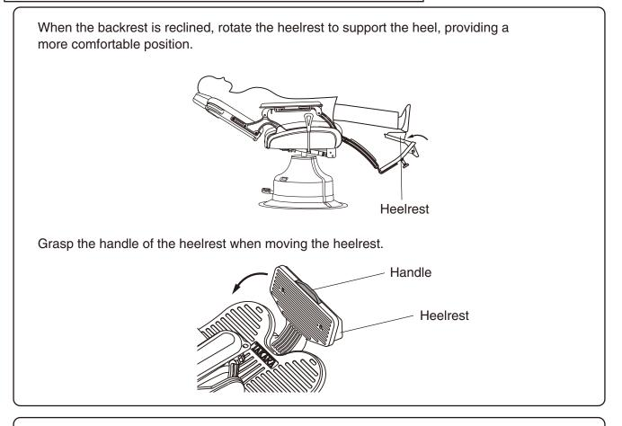
**CAUTION** Be sure to grasp the handle of the heelrest when moving the heelrest. Take care not to pinch foot of the customer or your finger in between the heelrest and step.
