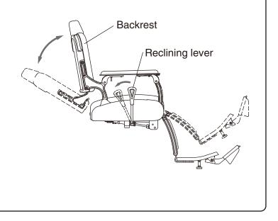
**CAUTION** When the reclining lever is tilted back, be sure to support and operate the backrest so that the backrest does not move suddenly.
