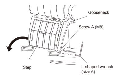
(2) Fold the step forward to fix it to the gooseneck using the screws and Screws A. (Fasten each of the four screws on the left and right sides similarly.)
