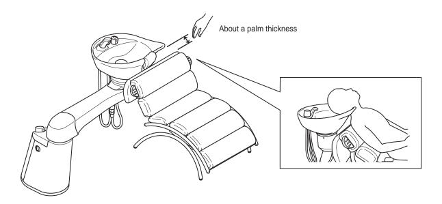
Adjust the shampoo position by sliding the seat back and forth with the headrest down and the seatback up.
