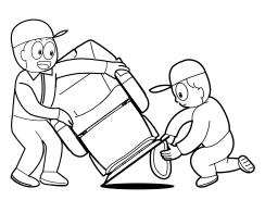
When it is difficult to carry the chair, attach the rubber ring or align the position while holding the base and foot switch, hold the armrest instead and perform the work. When doing so, pay attention to deformation of the cape holder, wrinkles and dirt of the leather, and coming-off of the base. Even if the armrest is held, the product may be damaged when excessive force is applied.
