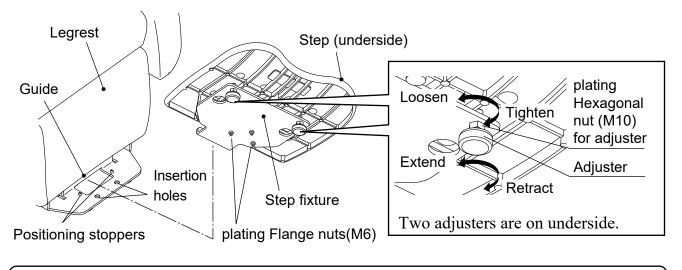
After installing the step, check that the step fixture is securely held by the guide, the plating Flange nuts(M6) are inserted in the insertion holes, and the step is not loose. Be careful that there is no looseness as this could result in instability when the customer is getting in and out of the chair, and in rubbing against the upper surface of the step when
