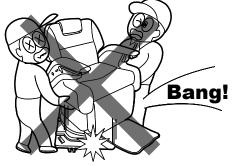
• Remove the chair from the skid. Raise the chair off the floor by holding up the metal plate under the foot switch. Move the chair by holding the base.
