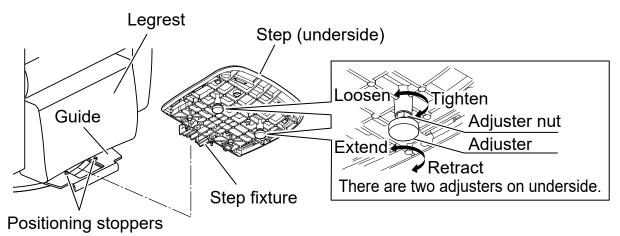
Insert the step at an angle (approx. 45°) and hook the step fixture on the guide while aligning with the positioning stoppers.
